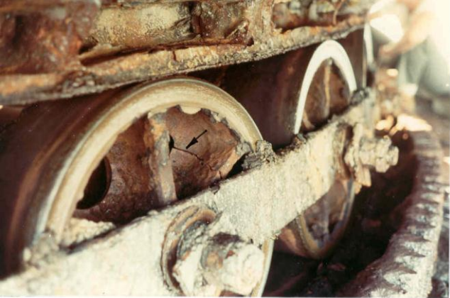
Figure 6.2.6.1i Rim support arrow - crack in wheel (note warp in upper track)
