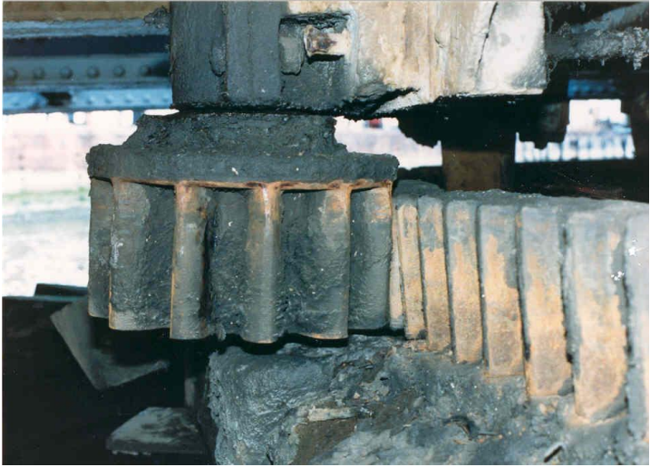
Figure 6.2.6.1i Rim support arrow - crack in wheel (note warp in upper track)
