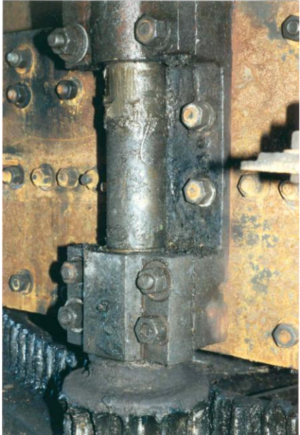
Figure 6.2.6.1l Journal bearings (top and bottom) - support for drive pinion assembly
