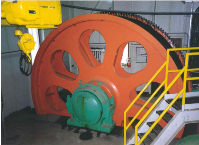
Figure 6.2.6.3g Sheave – bearing assembly tower drive Roller bearings
