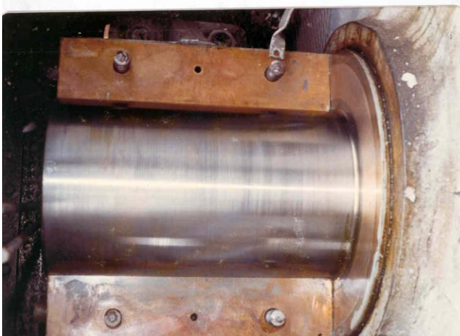
Figure 6.2.6.3g Sheave – bearing assembly tower drive Roller bearings
