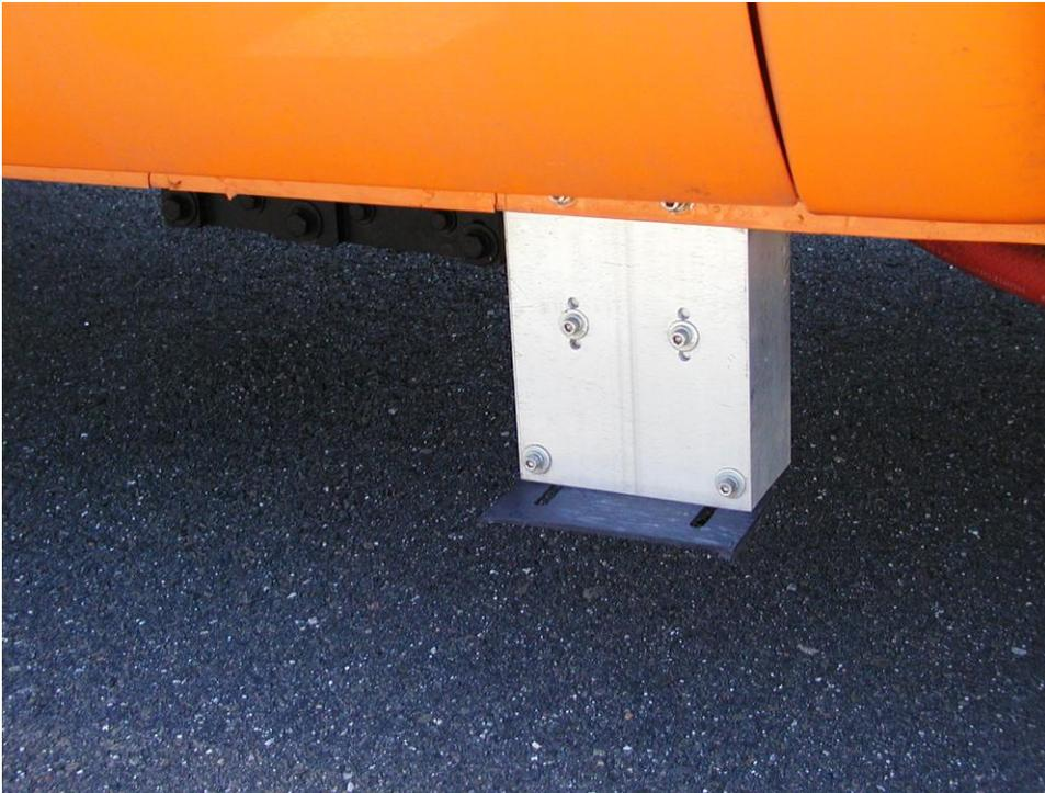
**FIGURE 2** Housing for High-Speed Selcom Optocator/SLS5000 Laser Sensor.
