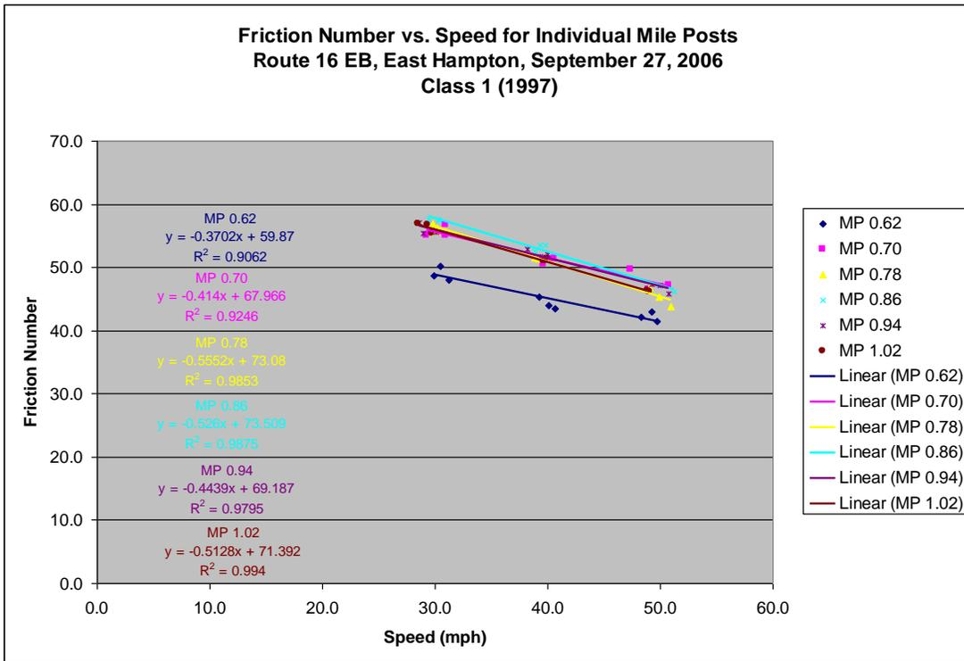
**FIGURE 13** Speed gradients at individual mileposts for Route 16 EB Class 1 pavement in East Hampton.
