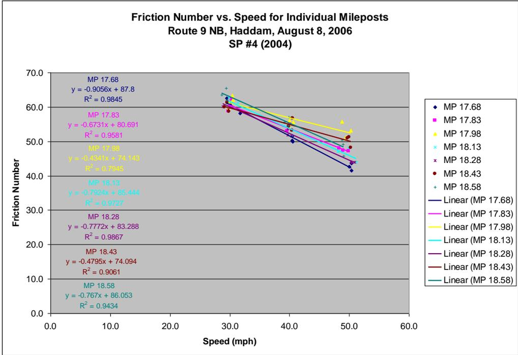
**FIGURE 31** Speed gradients at individual mileposts for Route 9 NB SP #4 pavement in Haddam.
