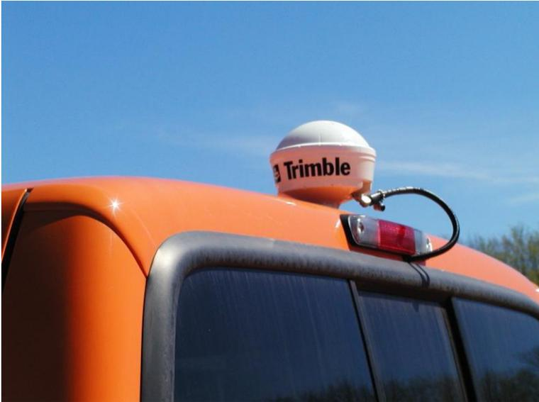
**FIGURE 3** Trimble Model AgGPS 33300-00 Global Positioning System.
