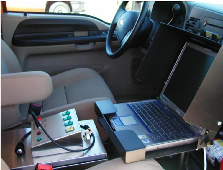
**FIGURE 5** Inside the cab of the Dynatest 1295 Pavement Friction Tester purchased in 2005.
