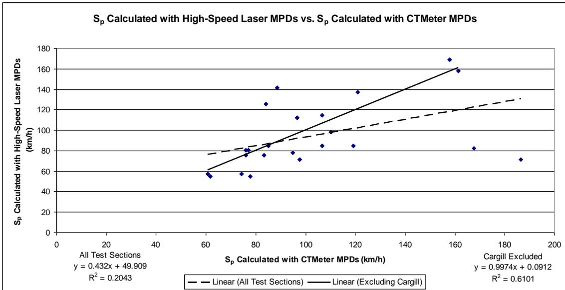
**FIGURE 53**  $S_p$  Values Calculated from High-Speed Laser MPDs versus  $S_p$  Values Calculated with CTMeter MPDs.
