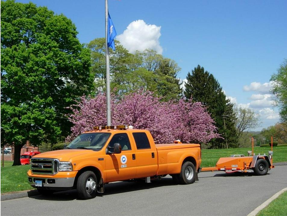
**FIGURE 1** Dynatest 1295 Pavement Friction Tester.
