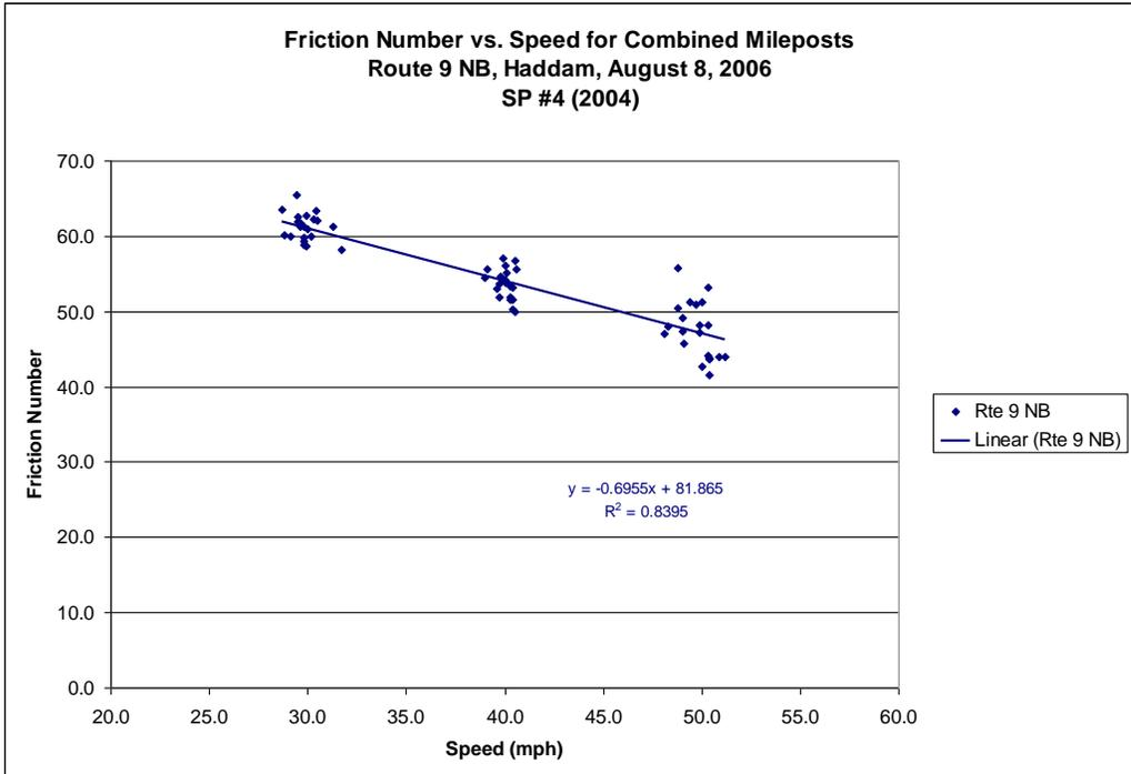
**FIGURE 32** Speed gradients combined for Route 9 NB SP #4 pavement in Haddam.
