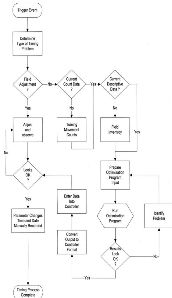
FIGURE 5 Classical approach to signal timing (Source: Henry 2005.)
