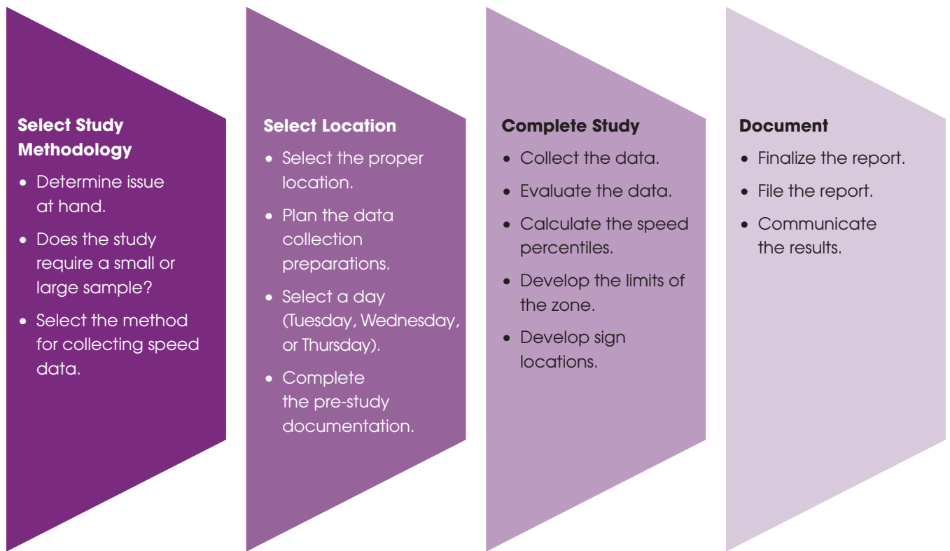
Figure 1. Speed Limit Study Process for Engineering and Expert Systems Methods.
