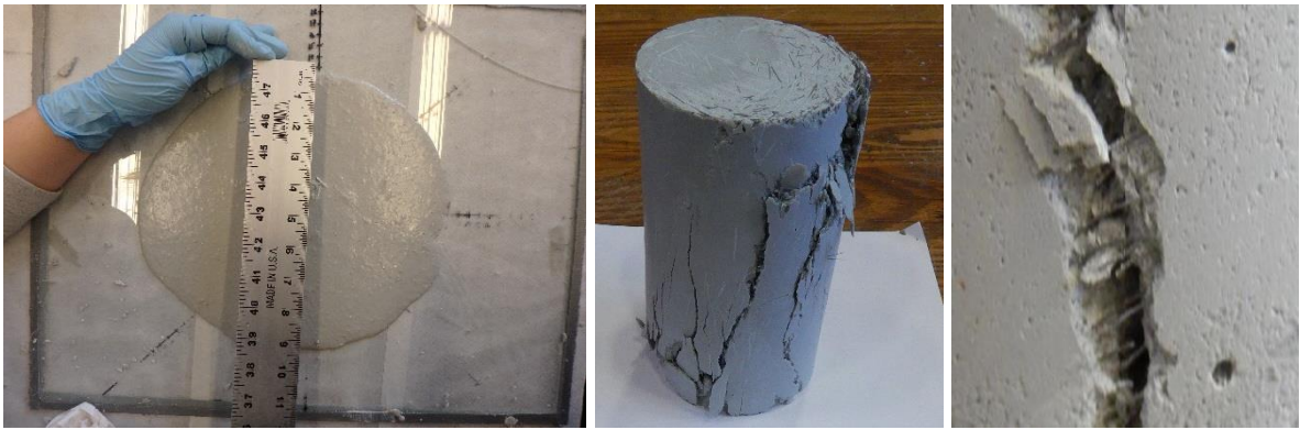
Figure 1.5: Material Testing of UHPC – a) good flowability, b) high compressive strength, & c) added tensile strength from steel fibers
