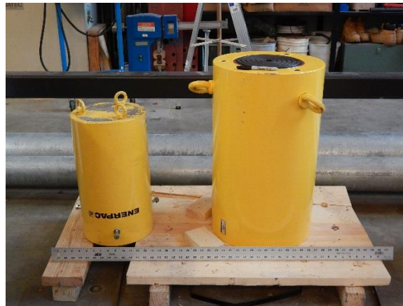
Figure 3.10: Enerpac CLRG-25012 (500-kip) and 50012 (1,000-kip) Hydraulic Cylinder
