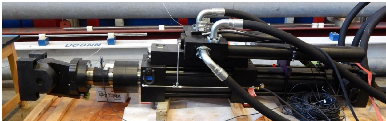
Figure 3.10: Enerpac CLRG-25012 (500-kip) and 50012 (1,000-kip) Hydraulic Cylinder
