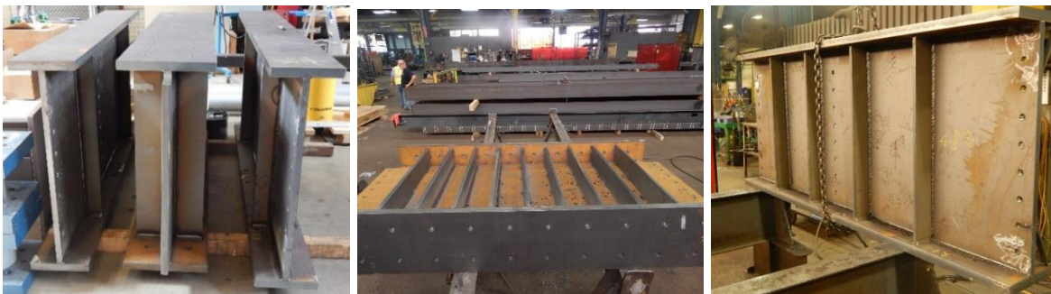
Figure 3.14: New plate girder spreader beams for the experimental test setup
