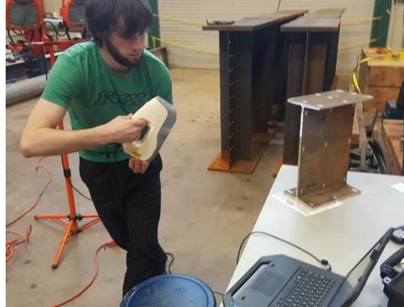
Figure 4.2: 3D Scanning using the Artec Eva
