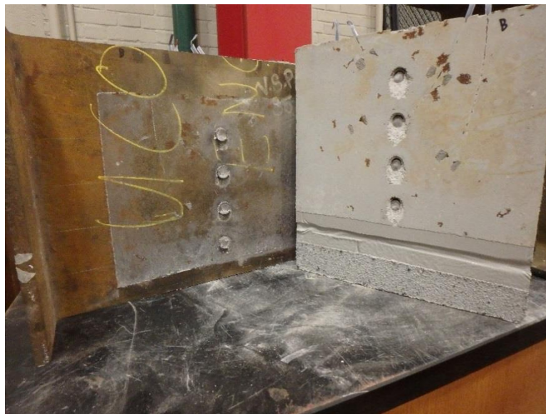
Figure 2.8: Typical failure of push-off specimen
