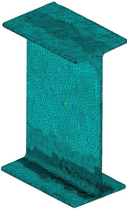
Figure 4.4: Finite Element 3D scanned mesh
