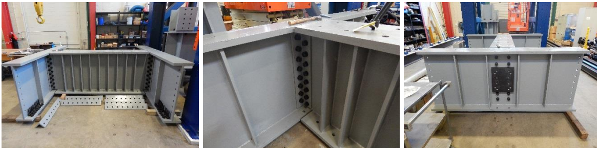
Figure 3.15: Load frame plate girder assembly with slip resistant paint
