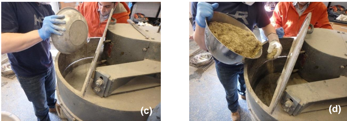
Figure 2.3: Mixing of (a) dry premix; (b) addition of water and superplasticizer,; (c) addition of chemicals; and, (d) addition of steel fibers
