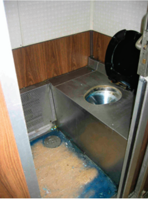
Typical M-4 re-circulating system
