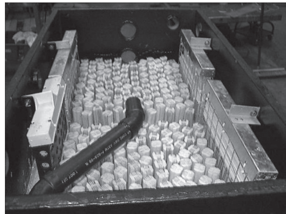
Microphor's redwood bark, left, and synthetic filter, right, for use in an on-board bacteriological waste management system.
