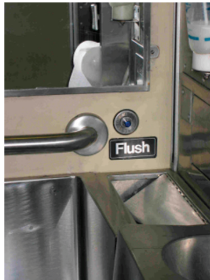
SPV Car (Shoreline East) - ADA flush control
