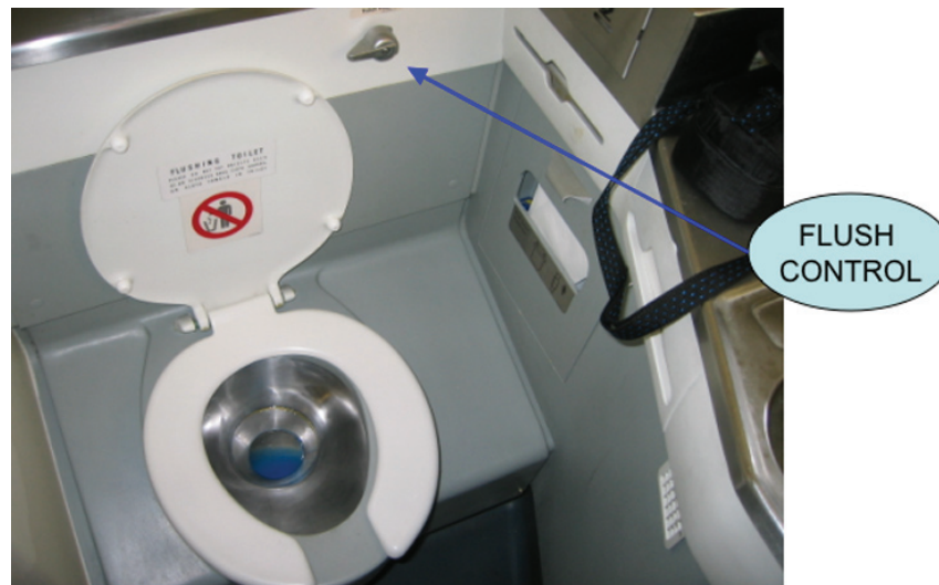
Example of re-circulating system (Southwest Airlines)
