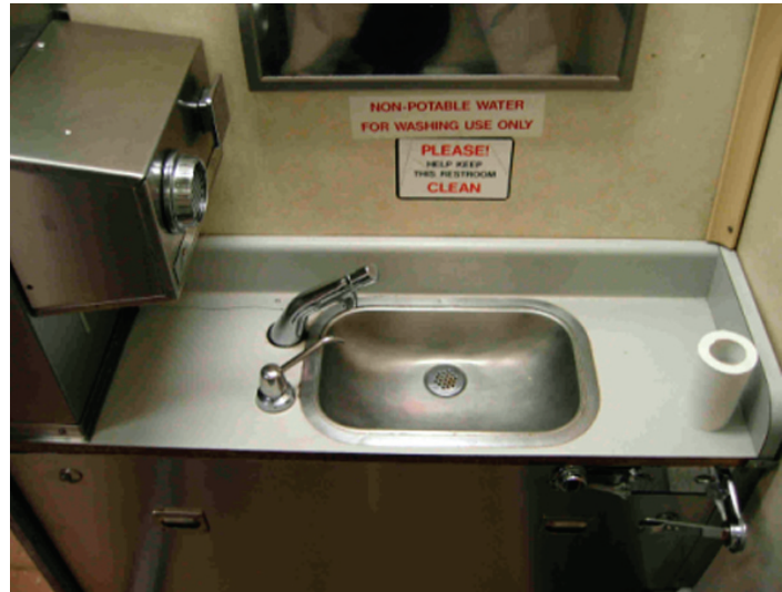
M-2 re-circulating system sink and counter
