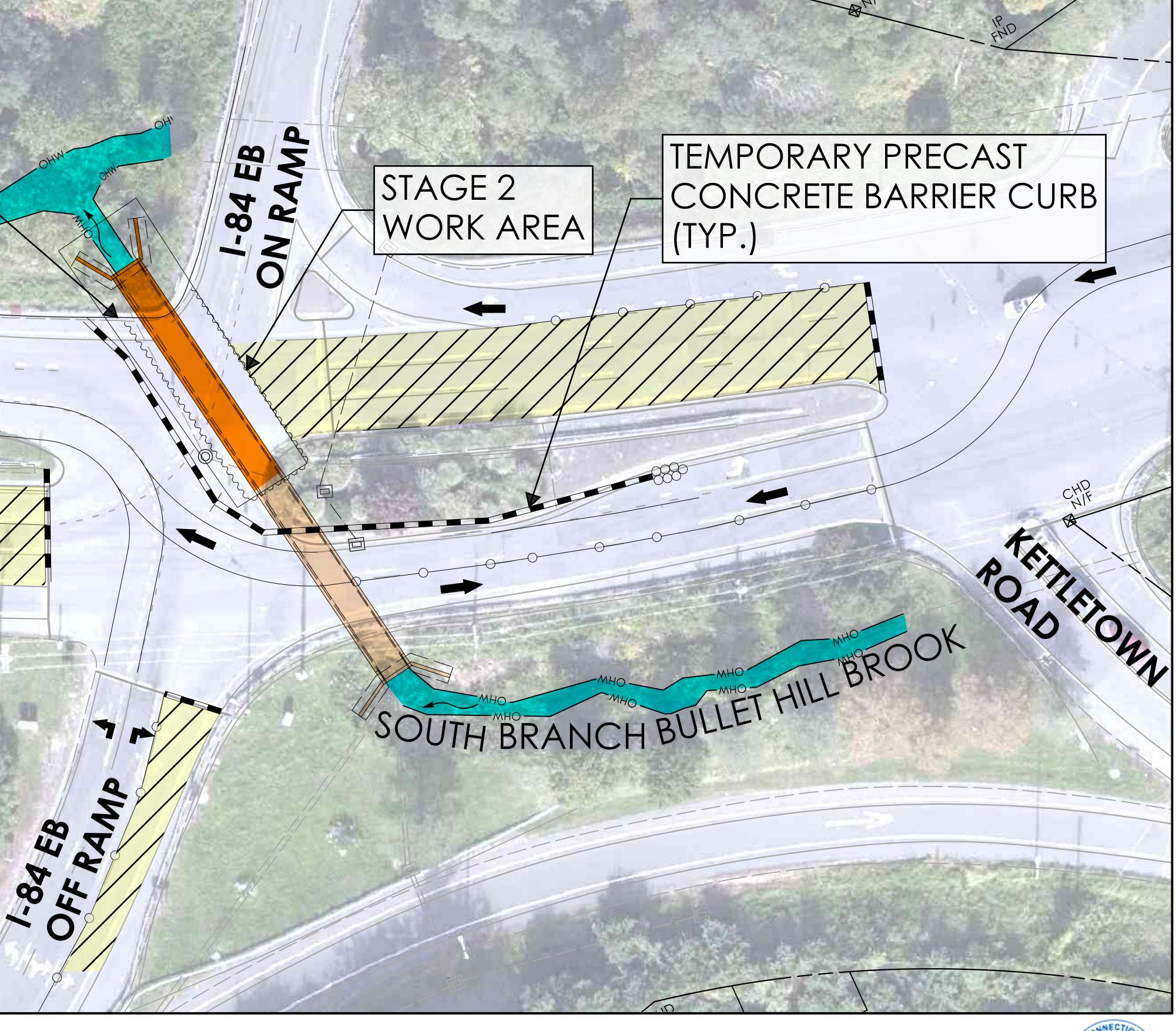
MAINTENANCE AND PROTECTION OF TRAFFIC - STAGE 2 US RT. 6 & SR 67 OVER SOUTH BRANCH BULLET HILL BROOK SOUTHBURY, CONNECTICUT
