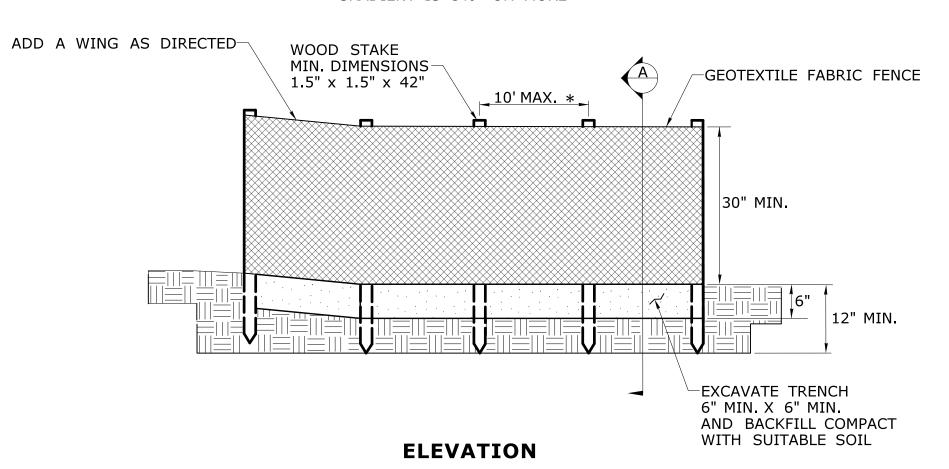
\* FOR SLOPES STEEPER THAN 2:1 USE A 5'POST SPACING OR AS DIRECTED BY THE ENGINEER
