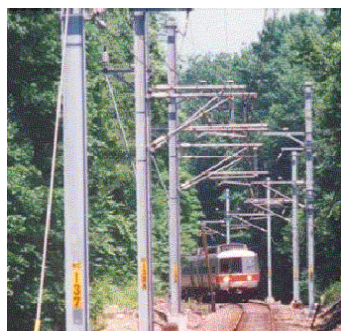
Example of electrified branch line: the New Canaan Branch with catenary poles and Electric Multiple Unit equipment.
