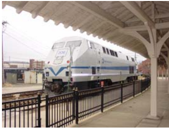
The Genesis locomotive is the primary diesel electric equipment currently used on the Branch.
