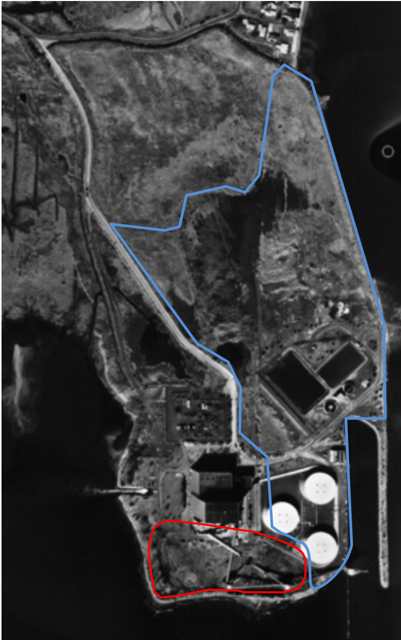
Figure 11: Manresa Island – 1985 Aerial Image. Approximate footprint of the former Manresa Institute identified in red. Note the areas of fill (identified in blue), as well as the new construction, including new oil storage tanks, associated with the CL&P power plant to the northeast.
