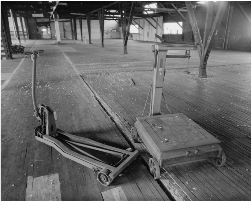
Some of the pier's equipment: a pallet truck (left) and a portable scale (right) (HAER photo by Robert Moore, 1993).
