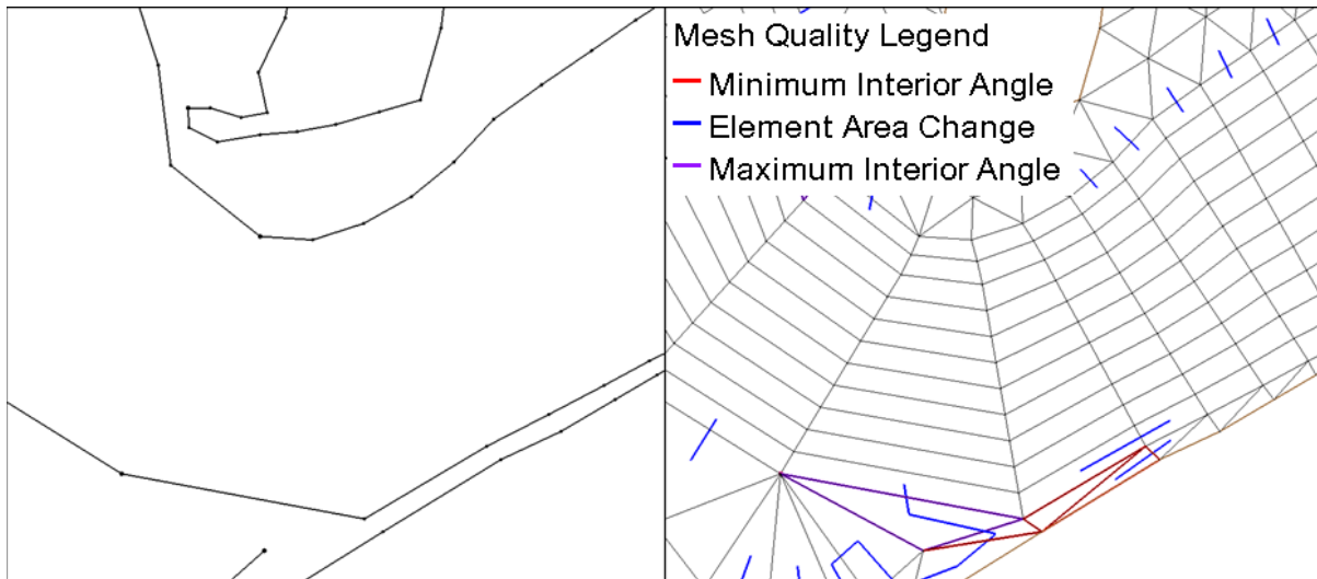
Figure 5.18. Element quality concerns in transition regions.
