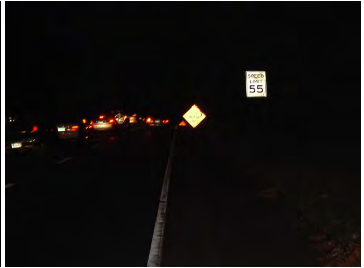
Again Mixed Sheeting types Bright Fluorescent (background) versus Type III first sign.
