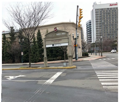
Figure 13: City Sign causing sight line issue
