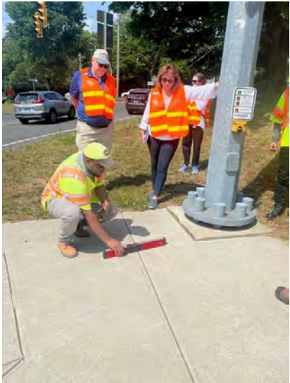
Exhibit 31: Sidewalk connection to the library doesn't exist on the northwest corner of the intersection (left). CTDOT's ADA team checking the slope at the northwest corner
