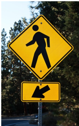
Figure 41. Example of Pedestrian Crossing with Down Arrow Sign at Uncontrolled Approaches
