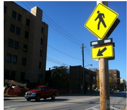
Figure 17. Pedestrian Warning (Rapid Flashing Beacon)
