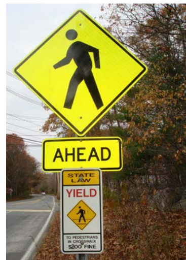
Figure 16. Pedestrian Advance Warning Sign
