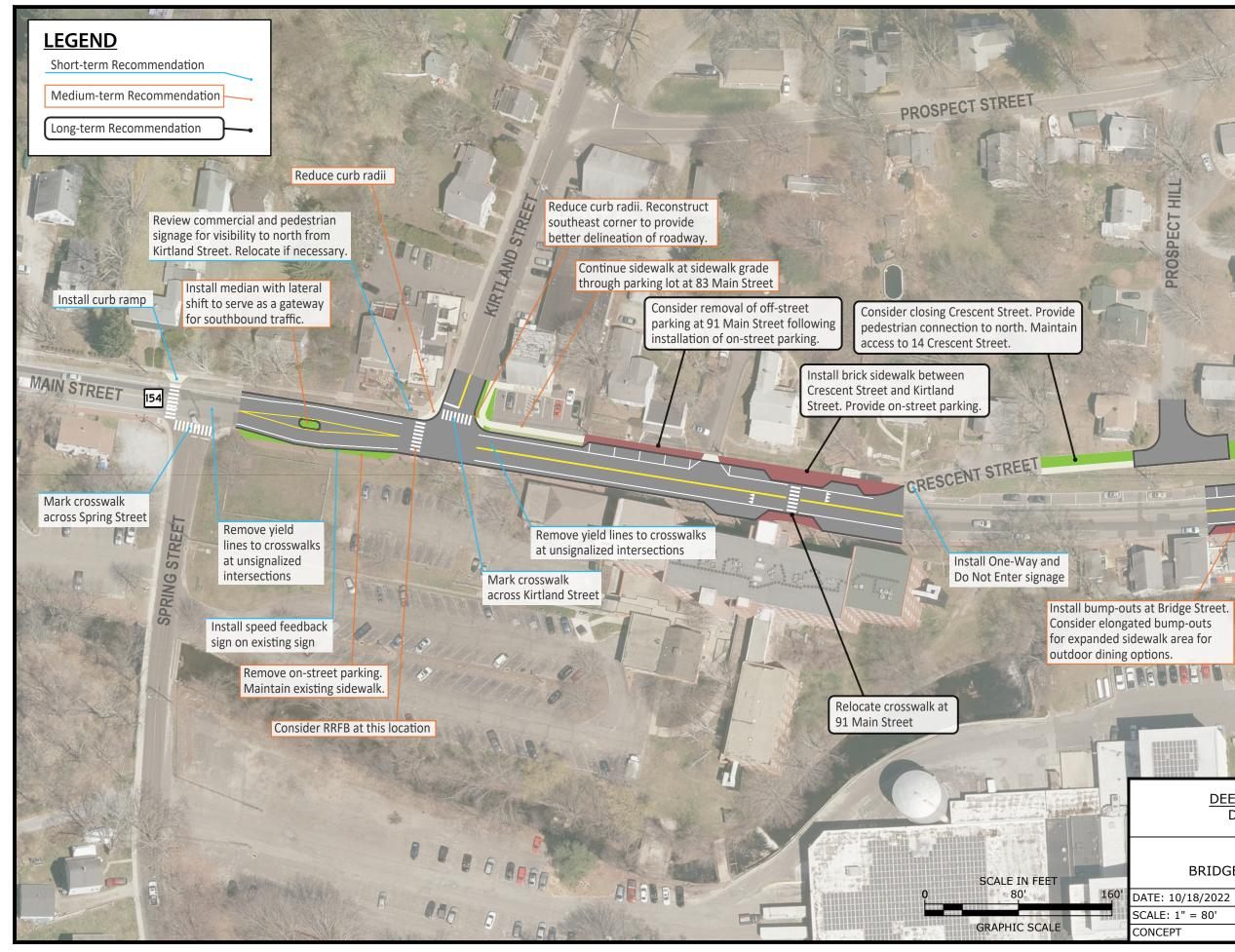
Install bump-out on east side to increase visibility to on-street parking to north. Relocate utility pole as necessary.
