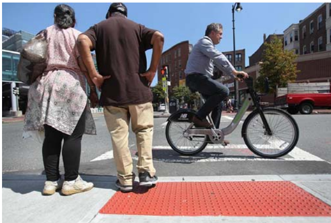
Figure 24. Example of Detectable Warning Strips
