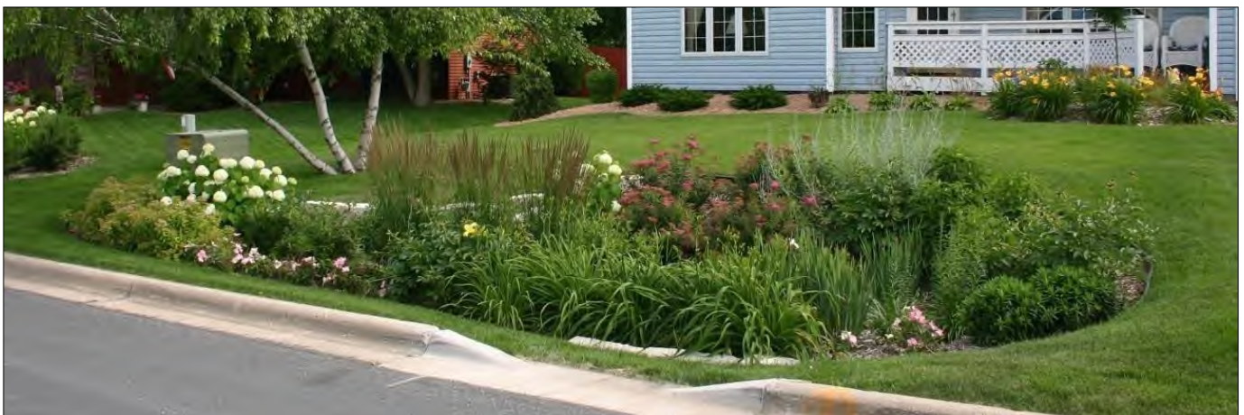
Rain garden for stormwater infiltration
