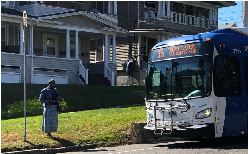
Exhibit 22: Transit rider waiting for Greater Bridgeport Transit (GBT) Route 15 bus at Route 1 and Judson Place. Note the limited accessibility at the bus boarding location and the lack of connection to the sidewalk
