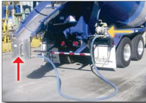
Figure 8. Chute washout bucket and pump
