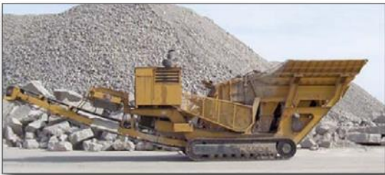
Figure 6. Crushed concrete stockpile and crusher
