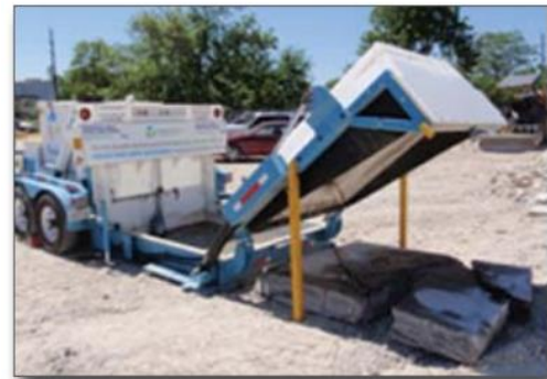
Figure 17. Delivering hardened concrete to a recycler
