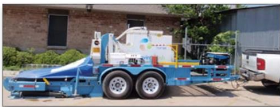
Figure 16. Washout container with a rain cover and onsite washwater treatment
