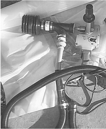
Drill shroud connected to HEPA vacuum: Collect dust where you're generating it.
