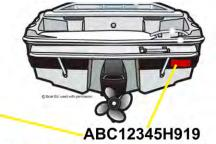
The HIN is typically located on the OUTSIDE of your boat, on the upper right hand corner of the transom. If your boat doesn't have a transom, like a canoe or kayak, then the number will be at the rear of the vessel, on the starboard (right hand) side, near the toprail. If your boat is a pontoon or catamaran, check the back of the starboard pontoon, or aftmost crossmember.
