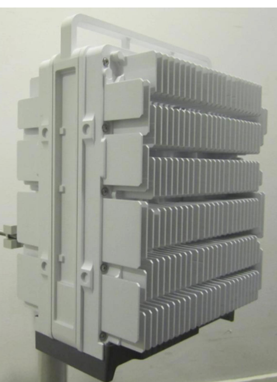
ERICSSON RADIO 4449 B12+B71 DIMENSIONS: 14.9"H x 13.2"W x 9.3"D WEIGHT: 74.0 LBS 1 PER SECTOR, TOTAL OF 3
