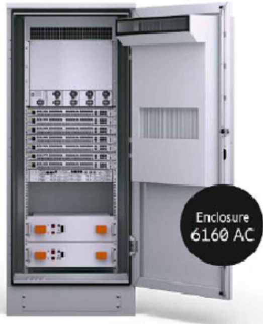
ERICSSON RBS6160 EQUIPMENT CABINET ENCLOSURE: ALUMINUM DIMENSIONS (HxWxD): 63" X 25.6" X 33.5" WEIGHT: 188LBS (EXCLUDES EQUIPMENT) WEATHER TIGHTNESS: NEMA TYPE 3R
