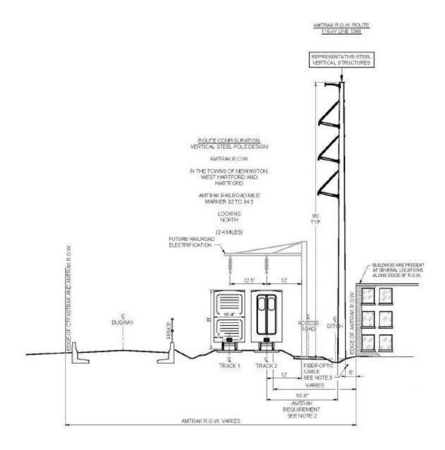
Attachment 4 – Typical Transition Structure Configuration (Eversource 1, Vol. 1, p. 3-12)
