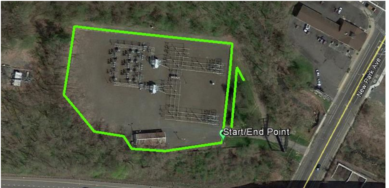
Figure C-4 – Measurement Path around Southwest Hartford Substation
