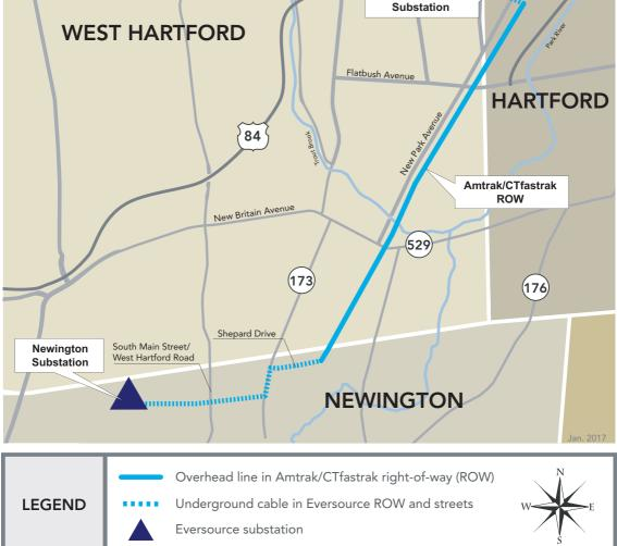
The map above shows the proposed route of the hybrid overhead and underground transmission line between Eversource substations in Newington and Hartford, as well as the substations where work will take place.
