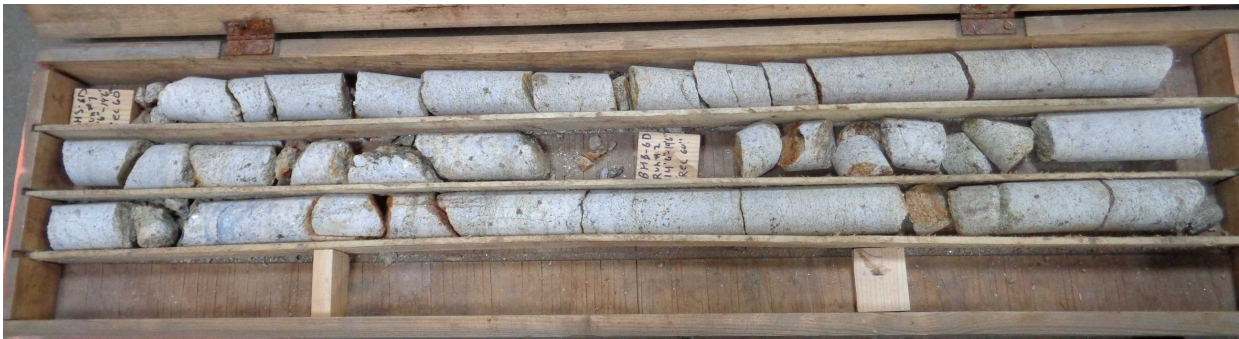
Boring BH-6D - rock core Run #1 taken from 9.5 to 14.5 feet and rock core Run #2 taken from 14.5 to 19.5 feet
