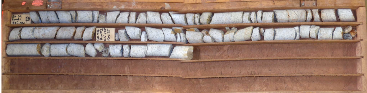
Boring BH-7A - rock core Run #1 taken from 7.5 to 12.5 feet and rock core Run #2 taken from 12.5 to 17.5 feet
