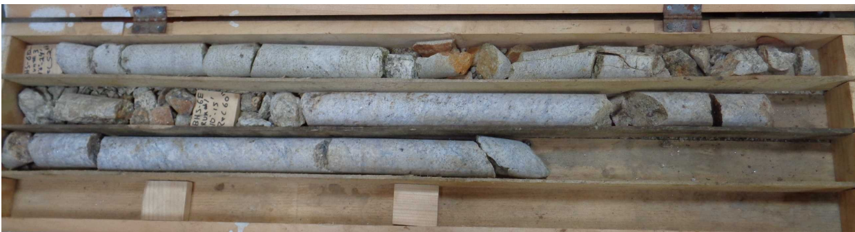
Boring BH-6D - rock core Run #3 taken from 19.5 to 14.5 feet; Boring BH-6E - rock core Run #1 taken from 10.0 to 15.0 feet
