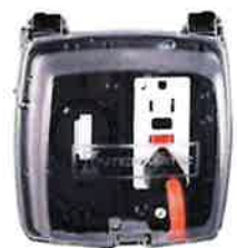
SWITCH DETAIL INTERMATIC WP122QC TYPE: DOUBLE GANG HINGE: VERTICAL INSERT: WP217 DEPTH: 2-1/4" COLOR: CLEAR OR APPROVED EQUIVALENT
