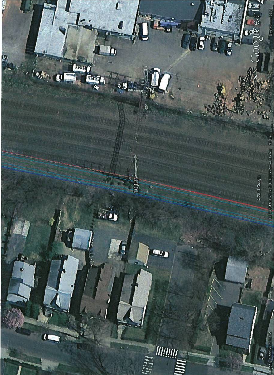
Location off of Scott Place near structure 1011. Tight construction and heavy side slopes. Large pads and ramps may be required.
