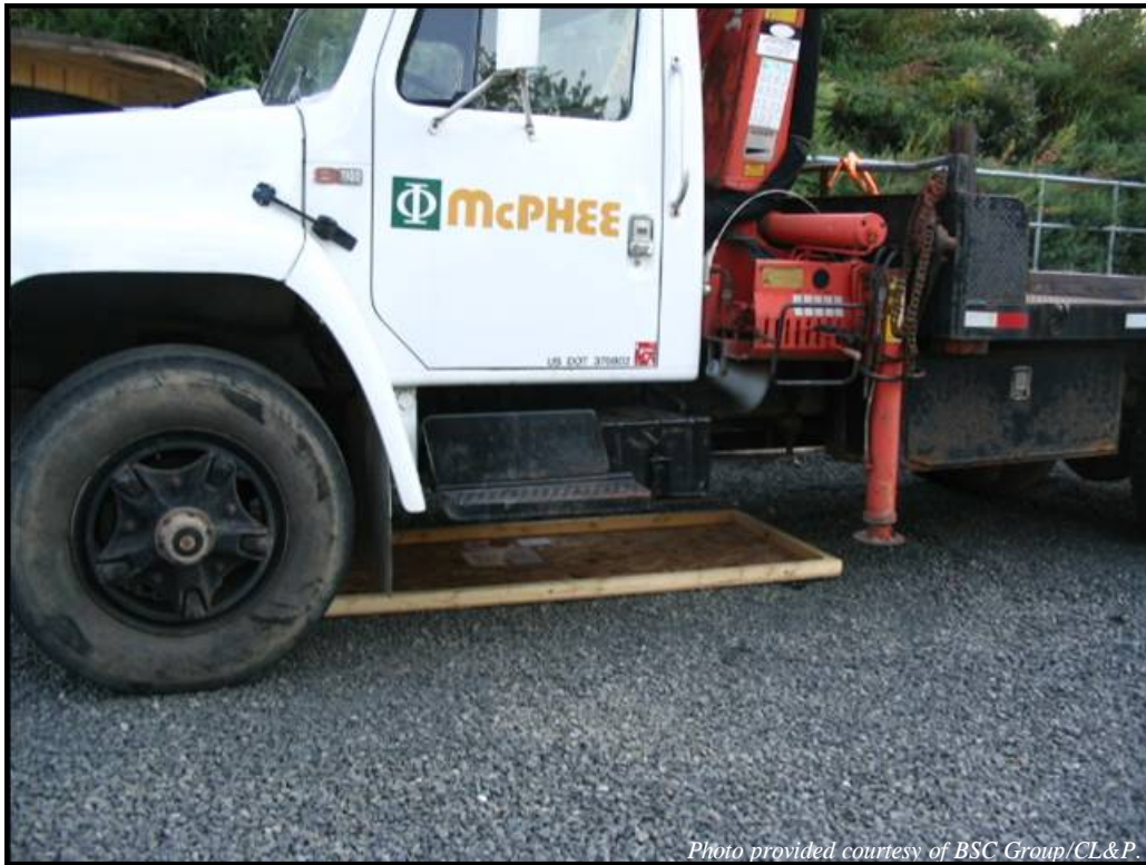
Photographs 11-2 and 11-3 Examples of good housekeeping practices (spill containment).
