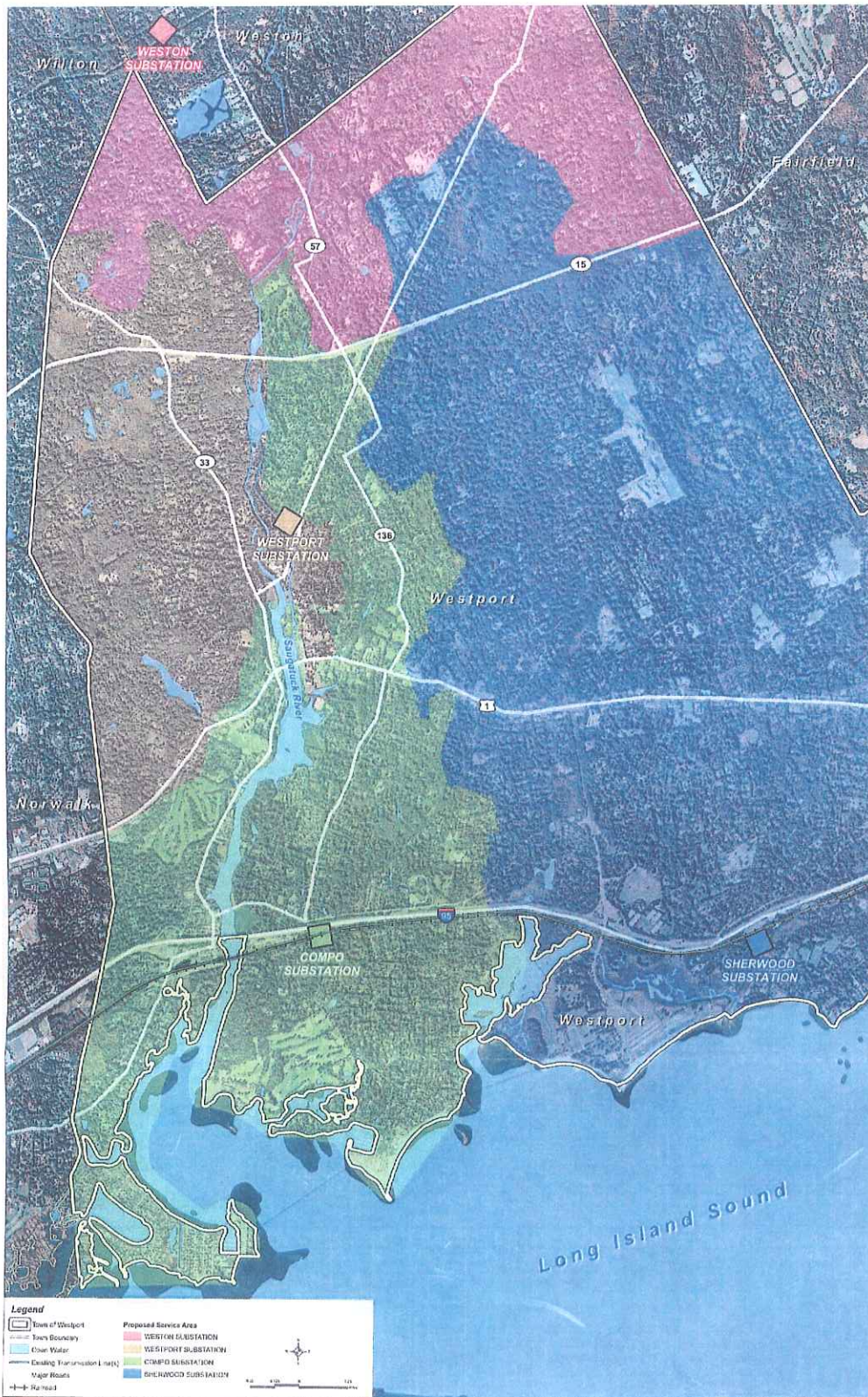
Figure 3: Westport Area Substation System after completion of proposed Sherwood Substation and removal of Green Farms Substation and temporary equipment at Sasco Creek Substation. (CL&P 1, Vol. I, Fig. G-2)
