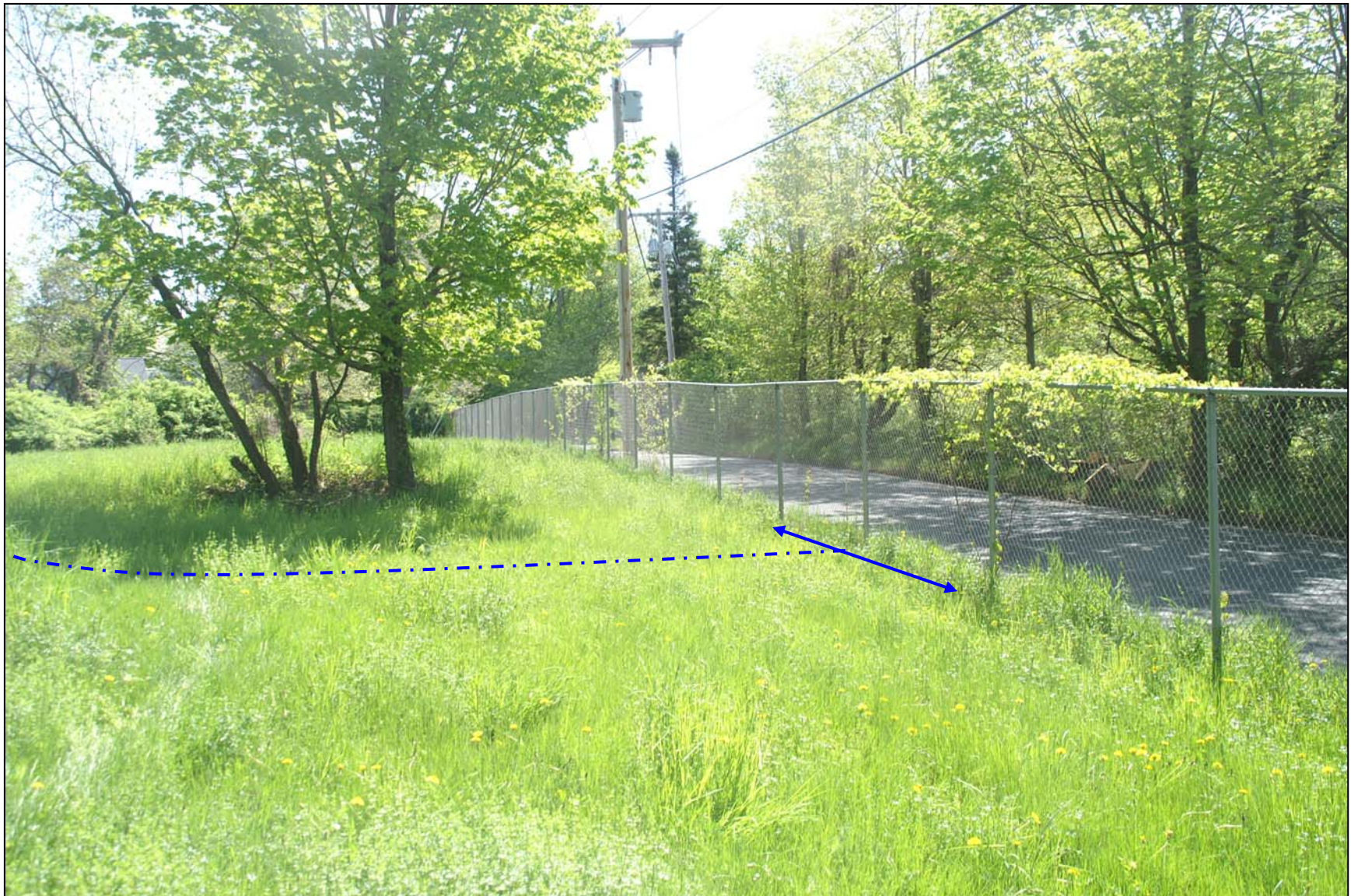
Photo 2– View from property looking east along Peck Road. Fence sections (indicated) to be replaced with turn in area and gate. Approximate centerline of access road indicated.
