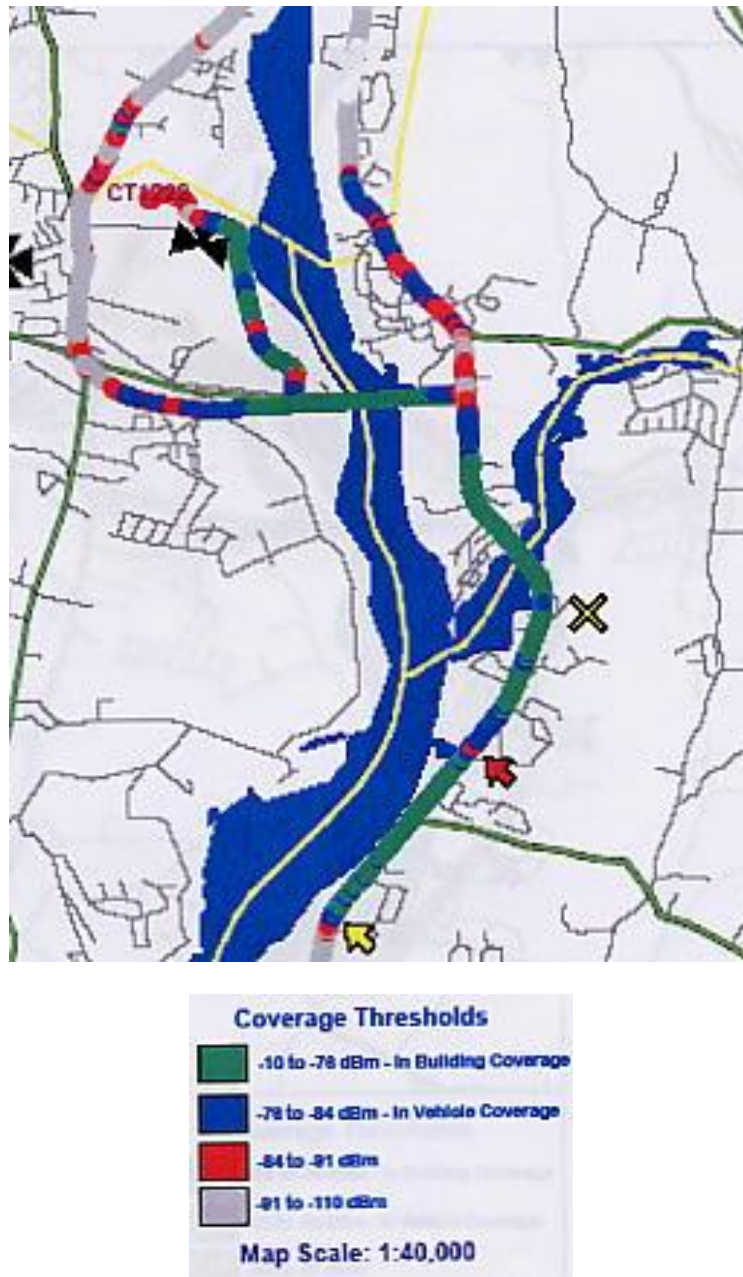
Figure 4. Drive test data showing expected coverage on Route 12 with antennas at 137 feet agl. The drive test shows 0.06-mile coverage gap (red arrow) south of the site (yellow X). The gap area would expand to 0.25 miles with antennas at 127 feet agl.
