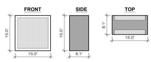
SAMSUNG DUAL LOW BAND B5/B13 (RF440d-13A) RRH 850/700 REMOTE RADIO HEAD (RRH) WxDxH=15.0"x15.0"x9.1" (82.0Lbs)
