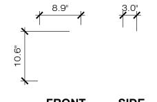
FRONT SIDE SAMSUNG CBRS RT4401-48A RRH HxWxD=10.6"x8.9"x3.0" (11.0 lbs)
