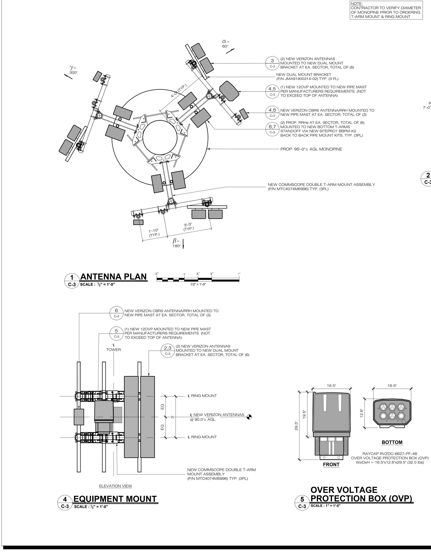
NEW VERIZON PANEL (3)ANTENNA TYP. (2PL) JMA WIRELESS MODEL #91900314-02 DUAL-MOUNT ANTENNA BRACKET P2.5 STD. (O.D. = 2.875") x 7'-0" LG GALV.ANTENNA PIPE MAST +
