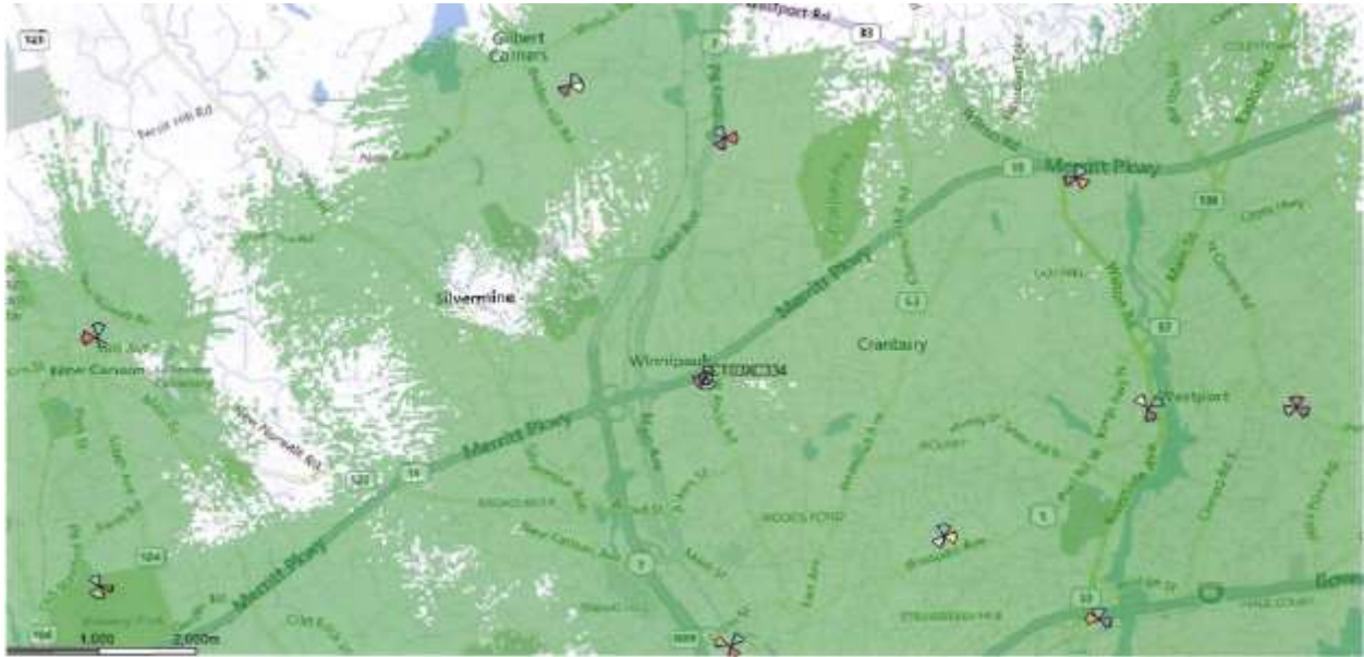
Figure 14 – Existing Sprint 1900 MHz Coverage with Existing Water Tank Facility
