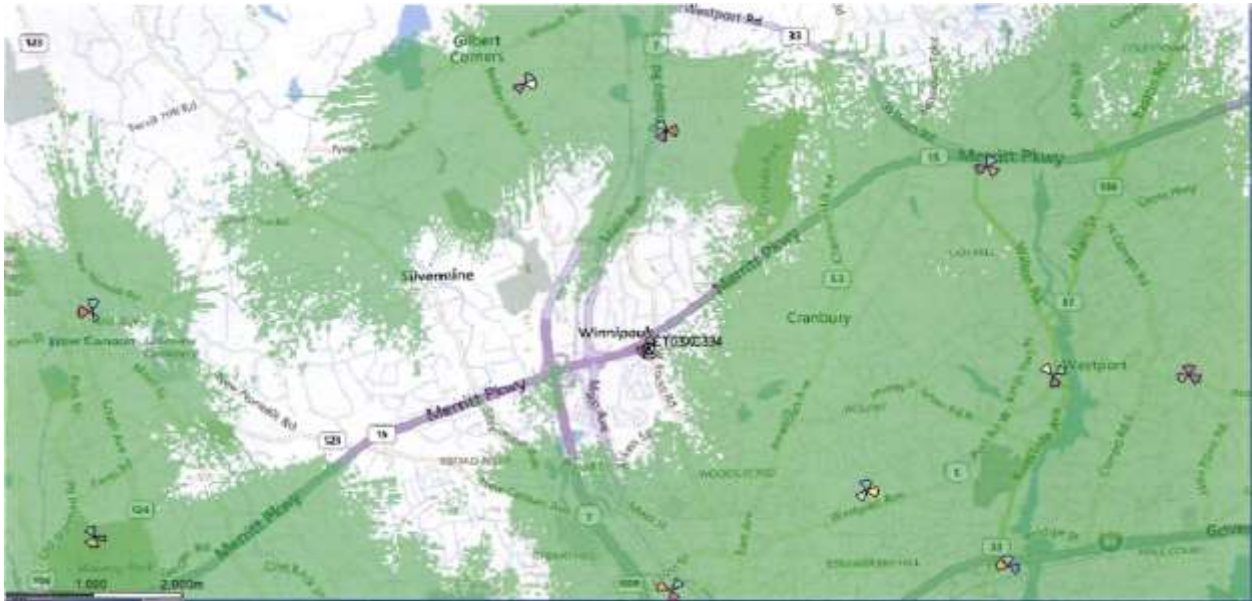
Figure 15 – Existing Sprint 1900 MHz Coverage without Existing Water Tank Facility
