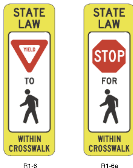
Figure 5-11. In-road pedestrian signs.
