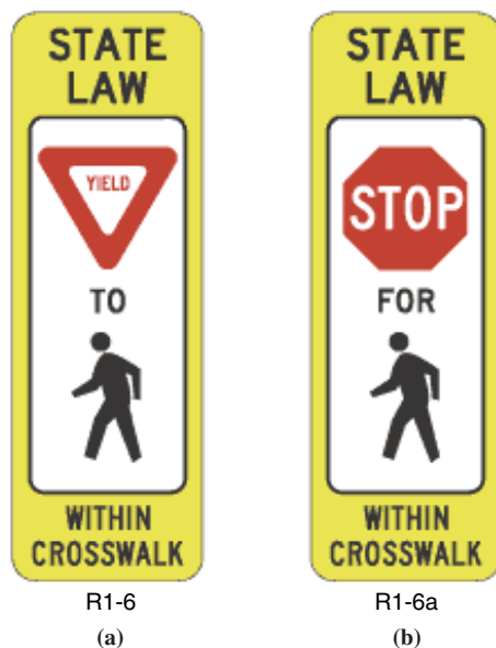
Figure 4-27. In-road pedestrian signs.
