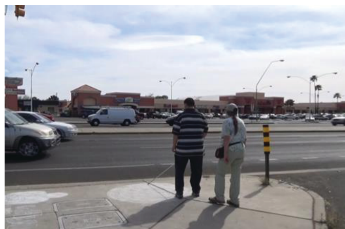
Figure 5-3. Blind pedestrian disoriented on an all-paved CTL island.
