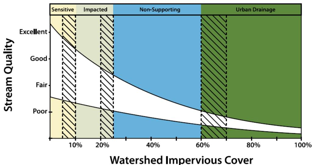
**Figure 6-3. Conceptual Model Illustrating Relationship Between Watershed Impervious Cover and Stream Quality**
