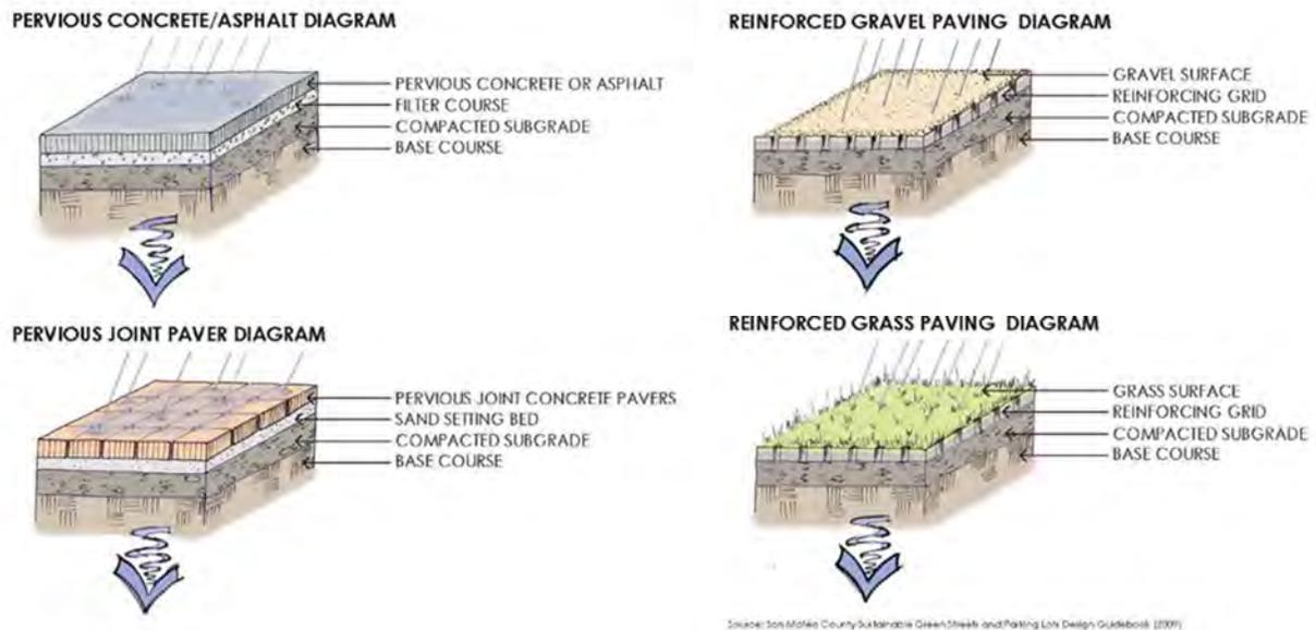
Figure 2.3.2. Diagrams of Selected Permeable Pavement Systems
