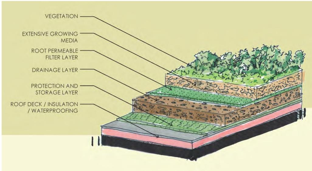
Figure 2.2.4. Typical Green Roof Design
