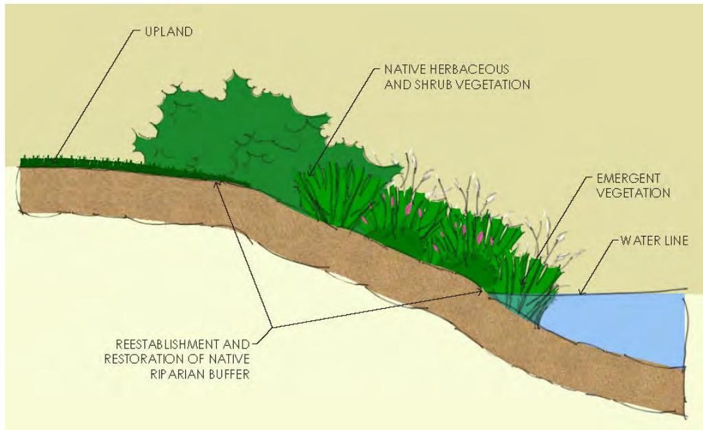
**Figure 2.6.3. Typical Bank Restoration Planting for Small Streams**
