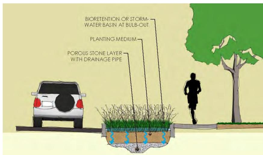
**Figure 2.4.3. Typical Green Street Bioretention Bulb-out**
