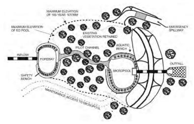
Source: Center for Watershed Protection. (2000). Maryland Stormwater Design Manual. Figure 2.7.2. Micropool Detention Pond Typical Design
