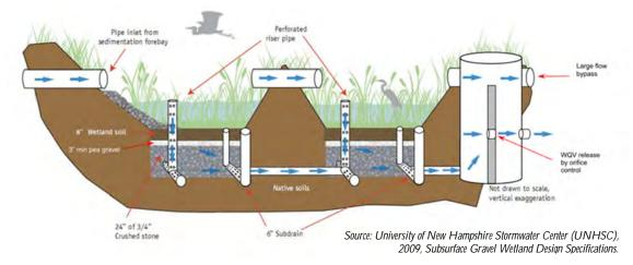
Figure 2.5.1. Typical Subsurface Gravel Wetland Design
