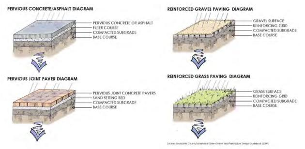
Figure 2.3.2. Diagrams of Selected Permeable Pavement Systems
