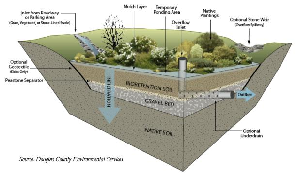
Figure 2.1.4. Typical Bioretention Design
