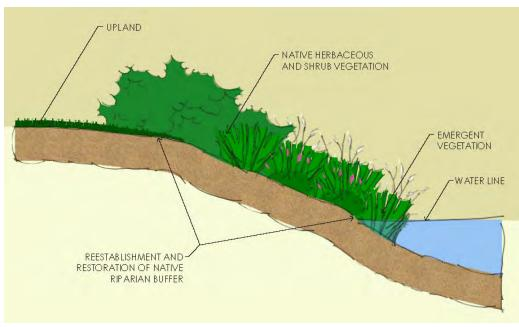
Figure 2.6.3. Typical Bank Restoration Planting for Small Streams
