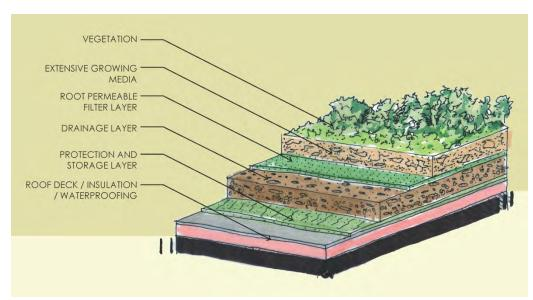
Figure 2.2.4. Typical Green Roof Design
