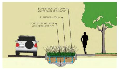
Figure 2.4.3. Typical Green Street Bioretention Bulb-out
