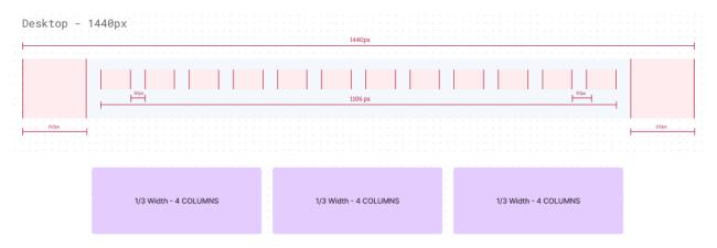
**3x3x3x3 Container:** this container divides the 12-column grid into 4 available containers each 3 columns wide. 3+3+3=12
