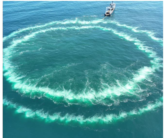
ThayerMahan, headquartered in Groton, deploys Hydrotechnik Lubeck Big Bubble Curtains that shield marine mammals from harmful construction noise. Aerial view of bubble curtain in action. Photo credits: ThayerMahan
