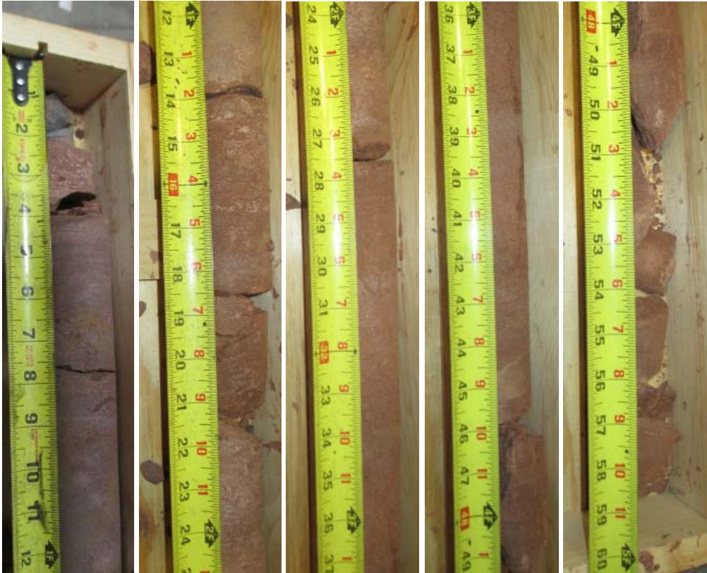
Figure 1. View of rock core extracted from 15' to 20' below grade (photographs altered to fit page).
