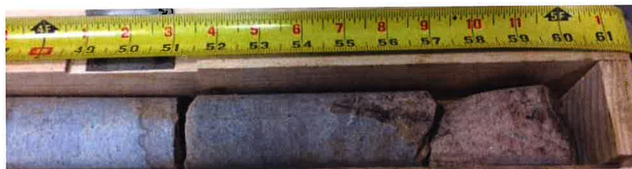
Figure 1a through 1e. View of bedrock core from 7 to 12 feet.
