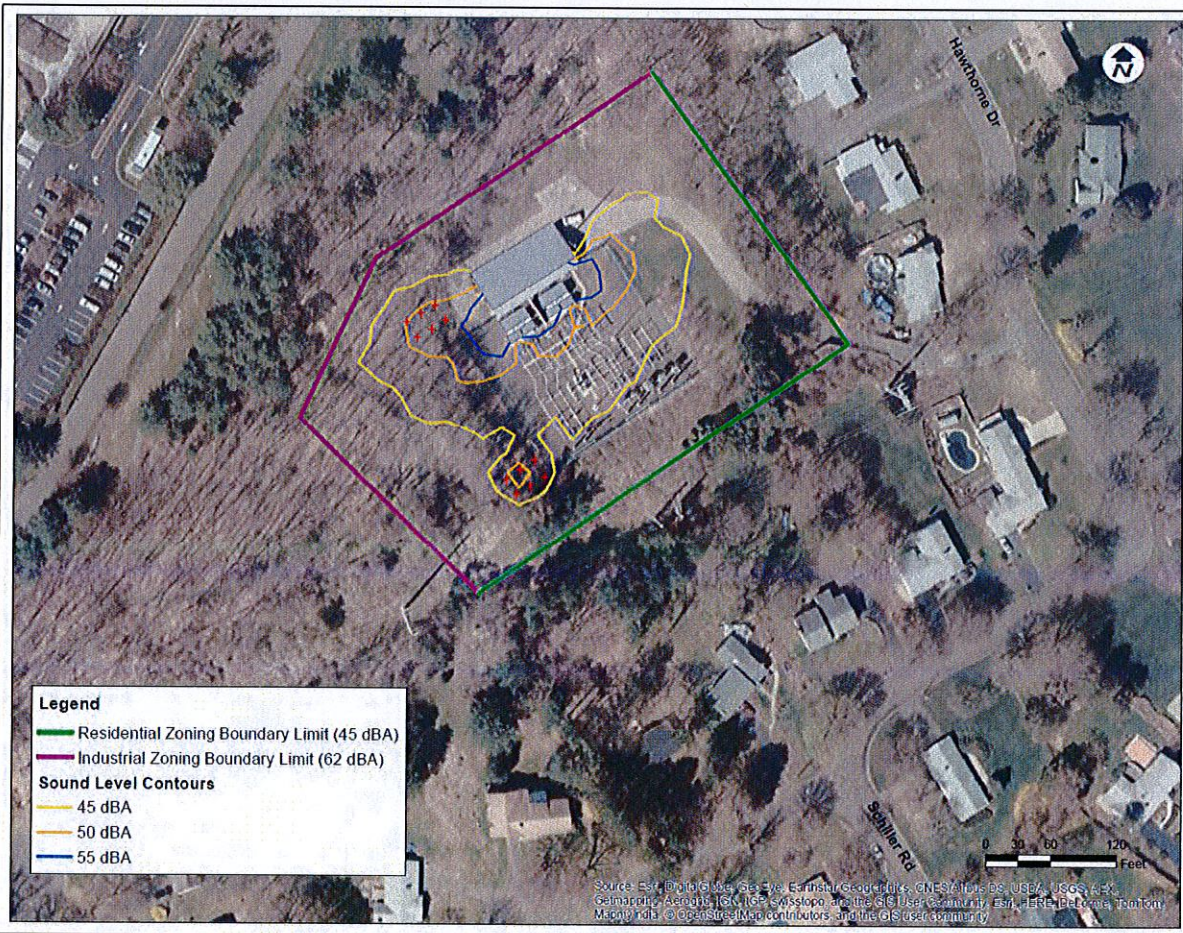
Figure 4-1 Future Substation A-weighted sound pressure levels, normal operation consistent with summer months.
