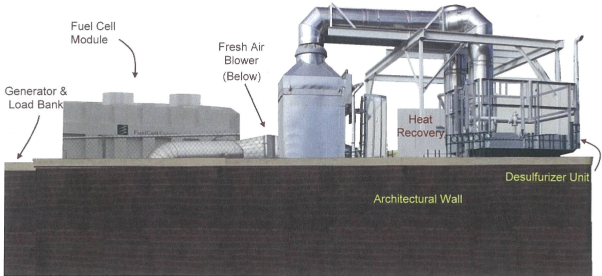
Figure 6: Annotated Model Summarizing of Individual Sources of Facility Sound with Solid Wall (shown as viewed from the south)
