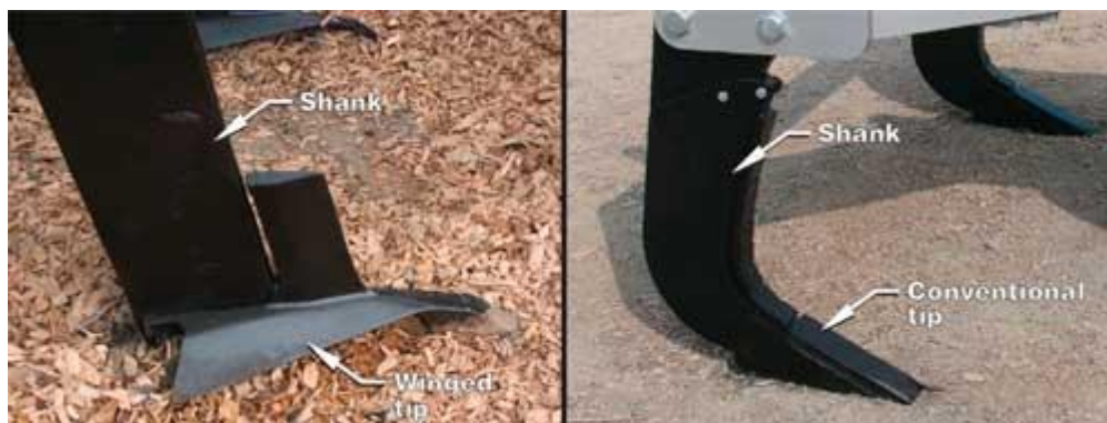
Figure 6.2: A winged tip and a conventional tip subsoiler (Kees 2008)
