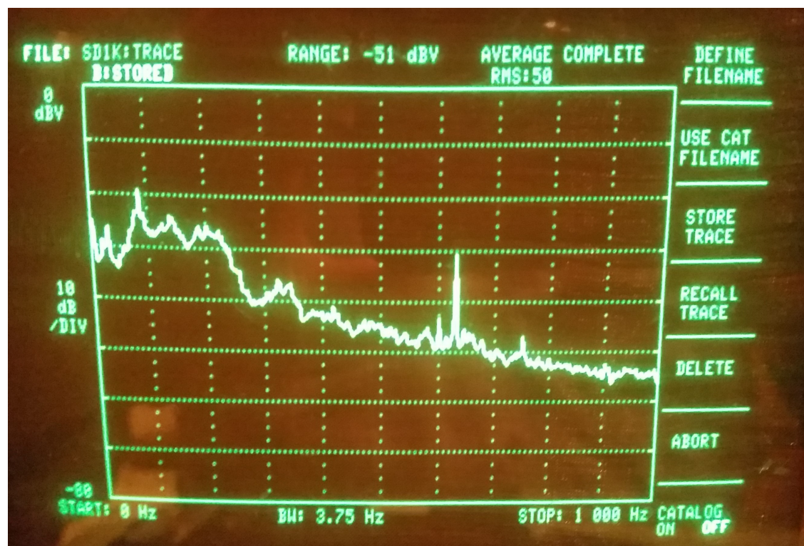
Figure 7. Discrete Tones Produced by Fuel Cell Cooling Module (0 dBV = 88.6 dB re20μPa)
