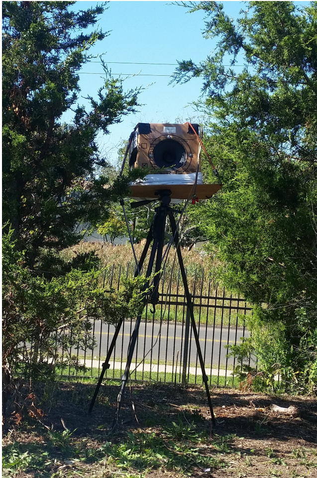
Figure 4. Speakers Used as a Simulated Airborne Noise Source at the Fuel Module Location
