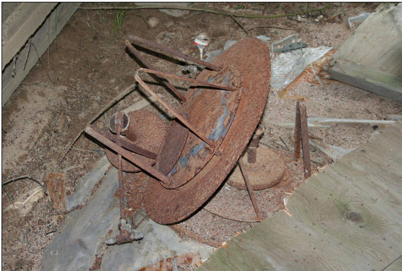
Photograph 75: Barn G (103), interior, detail of remnants of gas heaters.
